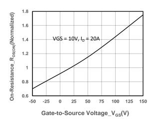
On-Resistance vs. Gate-to-Source Voltage
